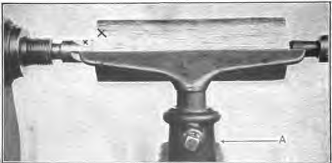
Fig. 9. Setting the Tee Rest.
